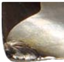
ER chuck wear detail
