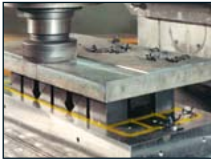
Milling warped stock with induction blocks
