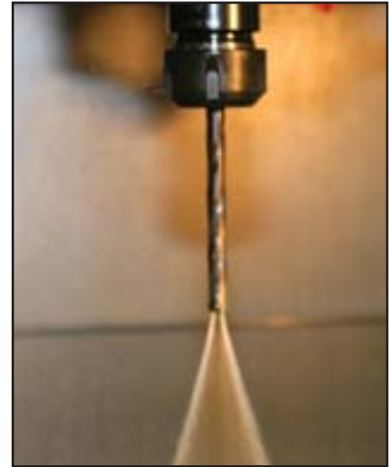
Use ER Coolant Rings with "o" ring for coolant-thru tool.
