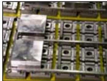
Machine induction blocks to create work-stops for fast, accurate part align- ment when ganging parts together for repeat jobs.
