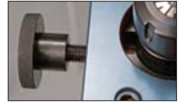
A large set-screw engages the drive slot in BT and CAT holders.
