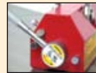
Lever in the "ON" position. The safety lock is engaged.
