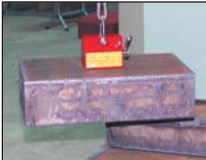
Center magnet on most workpieces to lift.
