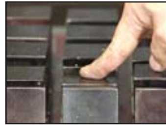
EEPM-SP50 spring-loaded for holding warped stock
