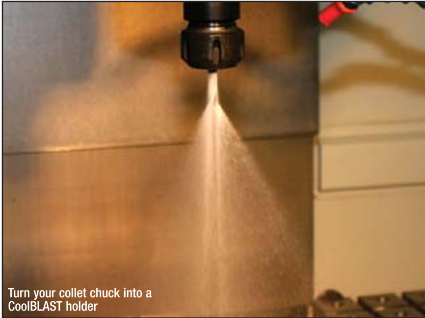
Use ER Coolant Rings with "o" ring for coolant-thru tool.
