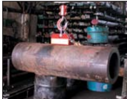
Beveled bottom surface lifts round stock.
